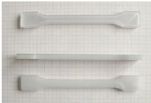
FIG. 3 3D printed test specimen tensile test
