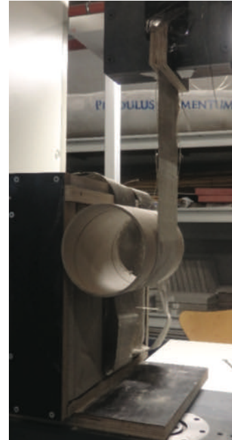
FIG. 8 Single-layer basalt fabric, test setup – peel-off test
