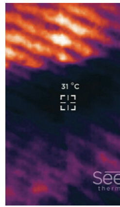
FIG. 8 Close-up of self-shading Thermal images of the surface in the inner area of the shading geometry Left: Shading range surface temp. 31°C ; Right: Exposure range surface temp. 36°C
