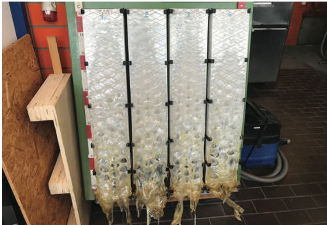
FIG. 6 Specimens lined up after the test for determining the residual length
