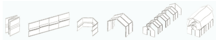
FIG. 20 zelthaus.com, research results from the PET area are used for self-supporting, insulated temporary buildings
