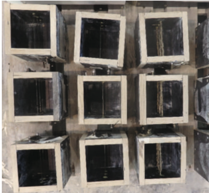
FIG. 7 Single rovings in form-work for pull-out tests
