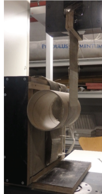
FIG. 8 Single-layer basalt fabric, test setup – peel-off test
