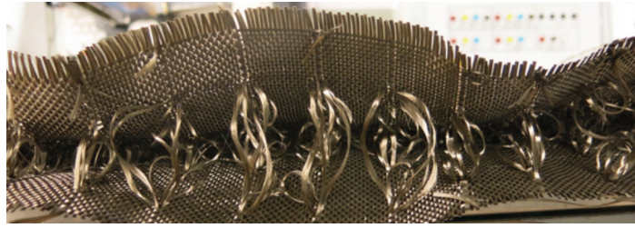
FIG. 12 First-time production of a double-curved spacer fabric made of basalt rovings
