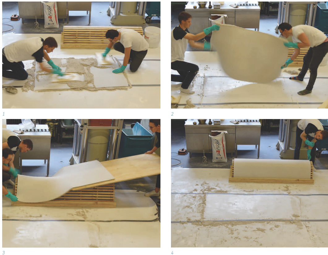
FIG. 14 Production of a form-active, single-curved component comprising an expanded glass/water glass matrix and a warp-knitted spacer fabric made of PE material: apply the material with a squeegee on one side of the cover surface, turn over, repeat the procedure on the other side; subsequent drying over a moulded part (alternatively, drying in a hanging position possible)
