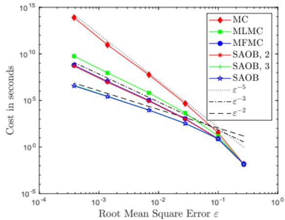
**Figure:** PDE example ( $\rho = 0.5$ ,  $\sigma^2 = 3$ ) with true cost rate  $\beta^{\text{Cost}} = 2$  (left image) and manufactured cost rate  $\beta^{\text{Cost}} = 6$  (right image). We can prove the complexity bound for the SAOB for the true cost rate  $\beta^{\text{Cost}} = 2$ , but not yet the complexity of the SAOB for the higher (manufactured) cost rate.
