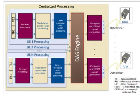
Fig. 1. Downlink shared channel transmitter processing chain adaptations for DAS
