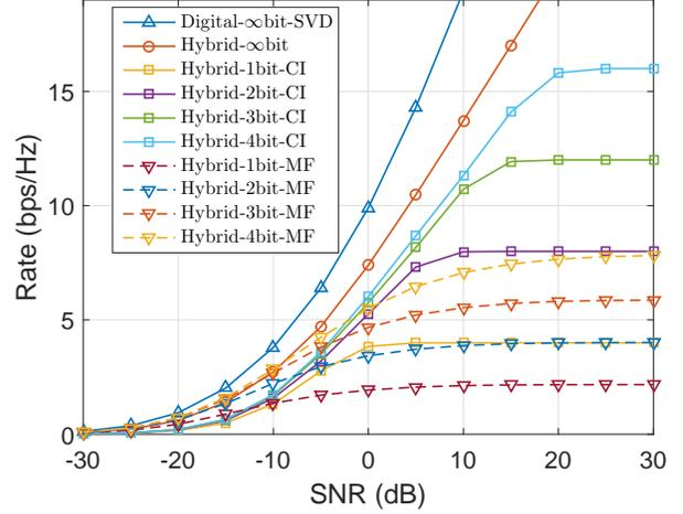
Fig. 2. Rates comparison of different receiver architectures when  $N_t = 16$ ,  $N_r = 8$ ,  $N_{RF}^t = 4$ ,  $N_{RF}^r = N_s = 2$ .
