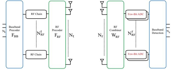
Fig. 1. A MIMO system with hybrid precoding and few-bit ADCs. Note that we assume the DACs at the transmitter have full precision.
