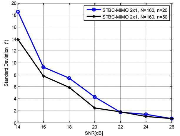
Fig.4. Standard Deviation of the novel phase synchronizer,  $N=160$ .
