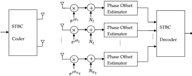
Fig.1. MIMO-STBC System with phase offset
