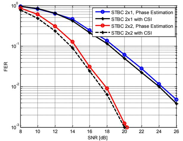
Fig.5. FER performance of STBC coded MIMO with phase estimation
