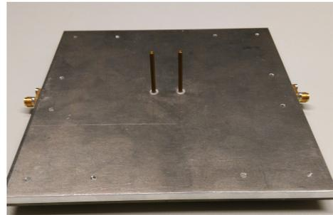
Fig. 1. Two-element monopole array
