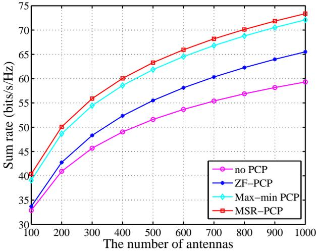
Fig. 3. Sum rate comparison of systems with various PCP techniques when users are randomly distributed in cells.
