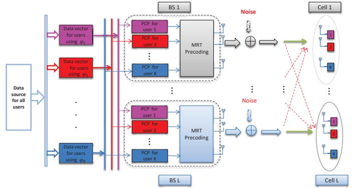
Fig. 2. System diagram with Pilot contamination precoding (PCP).
