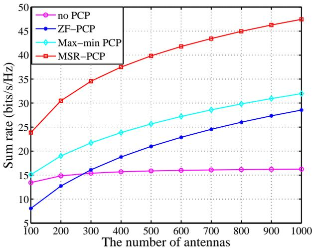
Fig. 4. Sum rate comparison of systems with various PCP techniques when users are located at the cell edges.
