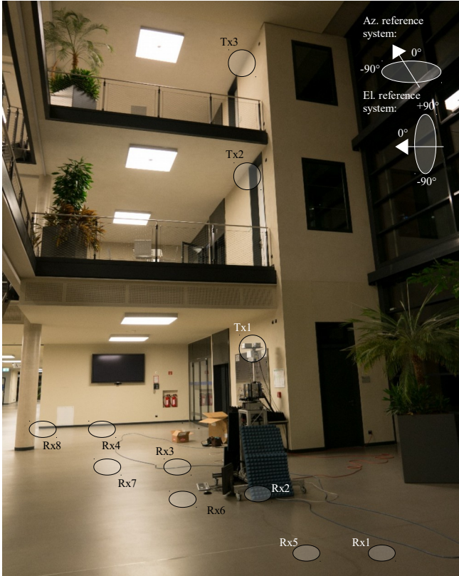
(a) Front view of the entrance hall. Position of the TX1, TX2, and TX3.
