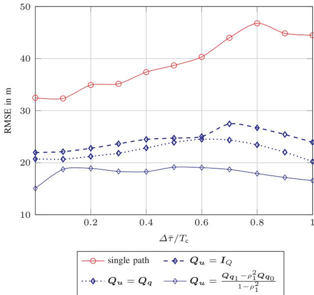
Figure 3. Estimation Performance of the CP Model for Different Choices of the Multipath Interference Temporal Covariance Matrix  $\mathbf{Q}_u$  over  $\Delta\bar{\tau}/T_c$  ( $L = 6$ )
