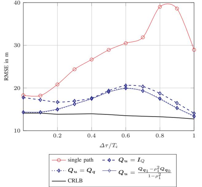
Figure 1. Estimation Performance of the CP Model for Different Choices of the Multipath Interference Temporal Covariance Matrix  $\mathbf{Q}_u$  over  $\Delta\tau/T_c$  ( $L = 1$ )
