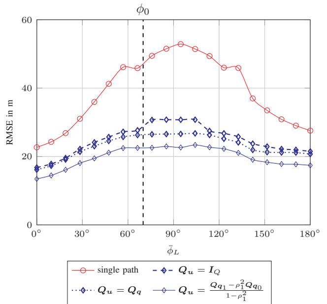
Figure 4. Estimation Performance of the CP Model for Different Choices of the Multipath Interference Temporal Covariance Matrix  $\mathbf{Q}_u$  over  $\bar{\phi}_L$  ( $L = 6$ )
