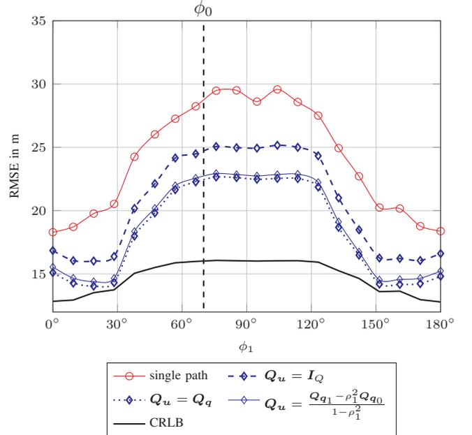
Figure 2. Estimation Performance of the CP Model for Different Choices of the Multipath Interference Temporal Covariance Matrix  $\mathbf{Q}_u$  over  $\phi_1$  ( $L = 1$ )
