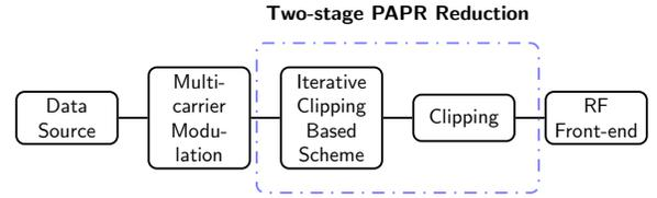
Fig. 5. Two-stage PAPR reduction scheme block diagram. In the first stage, one of the iterative clipping based schemes (i.e., TR, ACE, TRACE) is applied followed by a consecutive clipping at the second stage.
