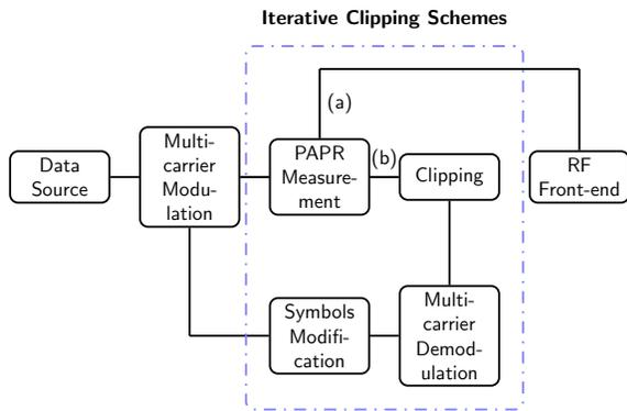
Fig. 3. Iterative clipping block diagram: the signal follows path (a) if the PAPR is less than or equal to the predefined threshold or if the maximum number of iterations set for the scheme is reached. Otherwise it will follow path (b).
