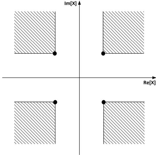
Fig. 4. Allowed regions for symbol extensions in a 4-QAM constellation diagram for active constellation extension (ACE).
