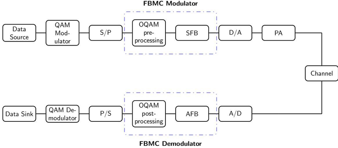
Fig. 1. FBMC/OQAM single-input single-output (SISO) transceiver structure based chain based on the PHYDIAS implementation [3] using synthesis filter bank (SFB) and analysis filter bank (AFB).
