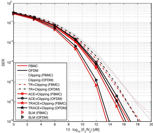
Fig. 8. Symbol error rate (SER) performance of OFDM and FBMC before and after the application of PAPR reduction schemes under investigation: for this figure, the number of sub-carriers is  $M = 64$ , oversampling factor of  $L = 4$ , the overlapping factor is  $K = 4$ , the prototype filter length is  $L_{\text{length}} = K \cdot M - 1 = 255$ , a constellation size of 4, and a clipping level of  $\text{CR}_{\text{dB}} = 3$  dB
