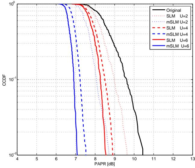
Fig. 7. Comparison of mSLM and SLM for different number of phase sequences  $U = 2, 4, 6$  for FBMC: for this figure, the number of sub-carriers is  $M = 64$ , oversampling factor of  $L = 4$ , the overlapping factor is  $K = 4$ , the prototype filter length is  $L_{\text{length}} = K \cdot M - 1 = 255$ , a constellation size of 4, and a clipping level of  $\text{CR}_{\text{dB}} = 3$  dB
