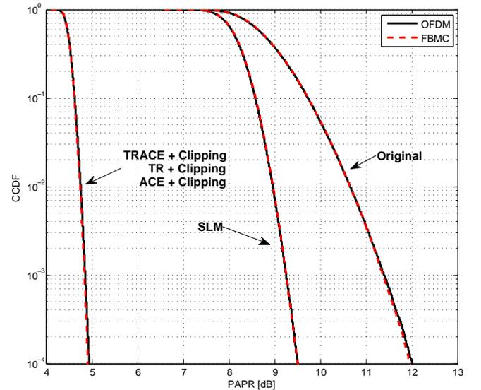
Fig. 6. Comparison of Two-stage (TR /TRACE /ACE /+ Clipping) and selective mapping (SLM) based PAPR reduction for OFDM and FBMC: for this figure, the number of sub-carriers is  $M = 64$ , oversampling factor of  $L = 4$ , the overlapping factor is  $K = 4$ , the prototype filter length is  $L_{\text{length}} = K \cdot M - 1 = 255$ , a constellation size of 4, and a clipping level of  $\text{CR}_{\text{dB}} = 3$  dB
