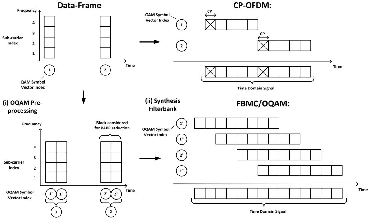
Fig. 2. Overlapping FBMC time symbols: for this example, the number of sub-carriers is  $M = 4$ , the overlapping factor is  $K = 2$ , the prototype filter length is  $L_{\text{length}} = K \cdot M = 8$  and number of QAM symbol vectors is  $n_{\text{symbol}} = 2$ .
